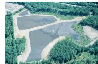
Hydraulic dredging containment area for Nutting Lake in Billerica – empty (above) and full (below)
