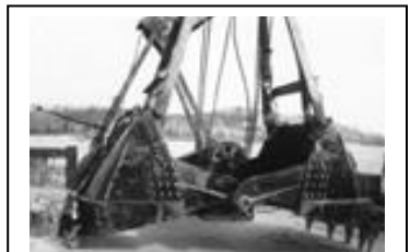
Clamshell dredge used in wet dredging operations
